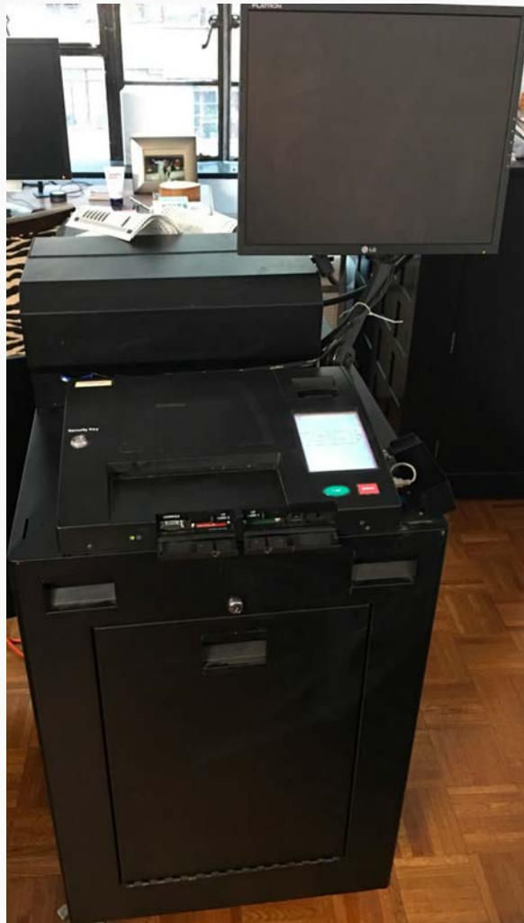
Picture: Dominion ImageCast Precinct with Ballot-Marking Device screen turned to face the scanner (back) side of the machine.
